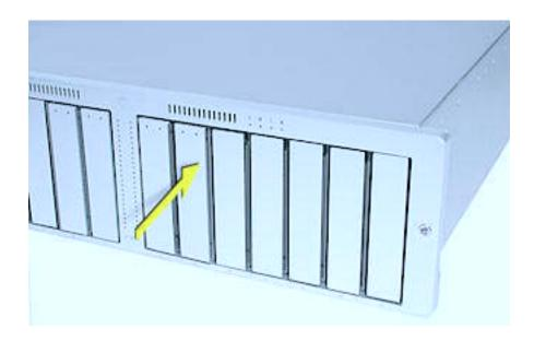
3. Wait for the right LED on the drive to go out. Then grasp the drive handle, and pull the drive module out of the system.
