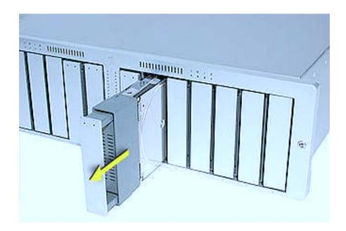
**Important**:To maintain proper airflow, do not leave a drive bay empty. If you permanently remove a drive, replace it with a blank drive module.
